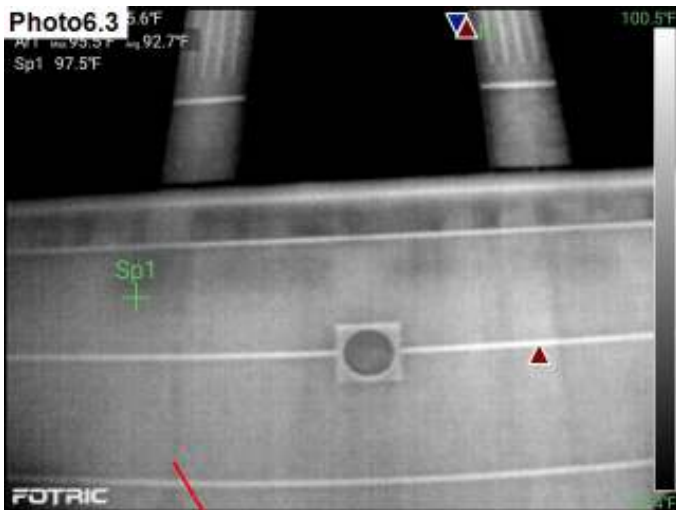
Front left side wall IR photo taken after sunset. The wall is not leaking; however, the windows are allowing moisture behind them to the inside drywall walls along the front left hall.
